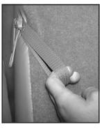
5. Pull up on the release lever labeled 1 and then pull up on the seatback or the assist strap located on the outboard side of the seat until the seatback locks into the upright position.
